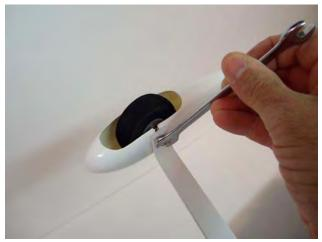
□□ **step 6**Hold the wheel pant parallel to the fuselage and drill the location for the wheel pant screw using a 1,5mm drill bit. Attach the wheel pant to the landing gear using a 2mm short self-tapping screw.
