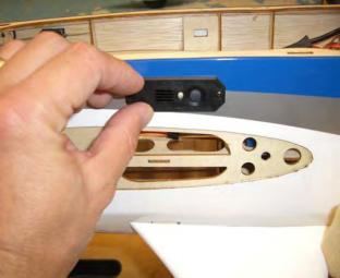
$\hfill \$  step 2 Locate and install the switch with a Phillips screwdriver as follow.
