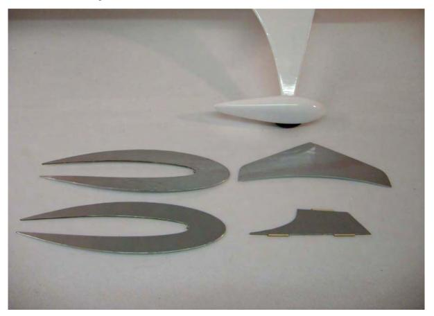
$\square$  step 2 Glue with medium CA the two parts of the fuselage's fin.
