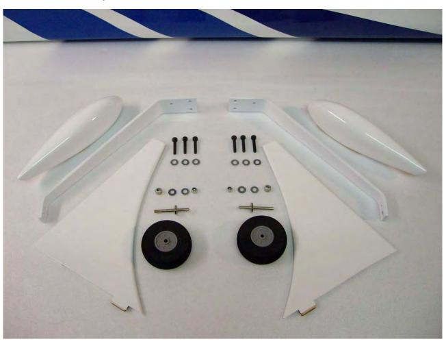
$\Box\Box$  step 2 Using screws and washers, install the landing gear as follow.
