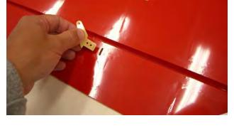
$\square\square$  step 4 Drill the location for the four self-tapping screw using a 1.5mm drill bit and install the servo into the wing panel using a Phillips screwdriver, as per the picture.
