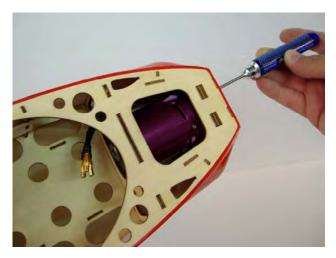
$\square$  step 4 Locate the plywood frame as motor support, and install it with self-tapping screws included in the hardware pack.
