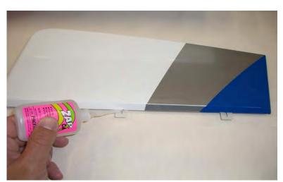
$\Box$  step 6 Carefully locate the rudder and glue the hinges with some drops of thin CA.
