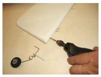
□ **step 4**Locate the tail wheel on rudder and glue it with some drops of medium CA.
