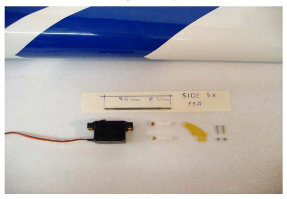
$\Box\Box$  step 2 With the hobby knife open carefully the servo location in the fuselage, as follow.
