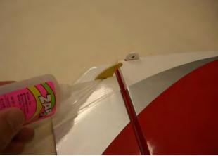
□□ **step 5**Install the elevator carbon tube, and using the provided two screws and washer install the stabilizer.
