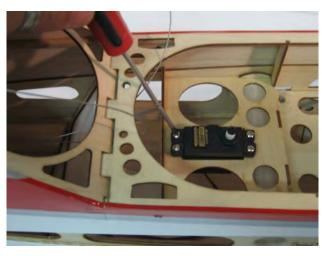
$\square$  step 3 With the hobby knife remove the cover on both rudder's side in the control horn location.
